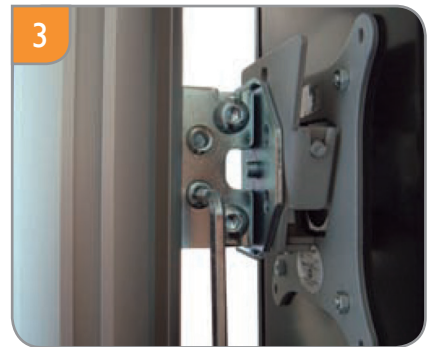
3 Adjust and tighten 4 screws at side of interface bracket until securely clamped to post in desired position.
