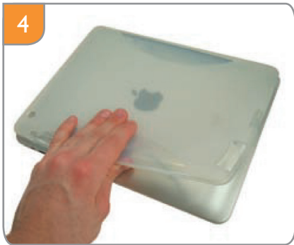
4 If using the iPad 2, 3 or 4 please insert the iPad into the silicon protective sleeve provided, to minimise movement within the enclosure.
