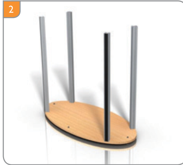
4 x Posts fitted into place.
