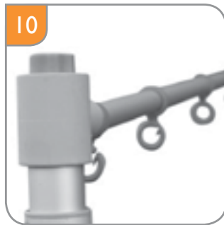
10 Affix support arm to top of pole and screw on nut to hold in place.
